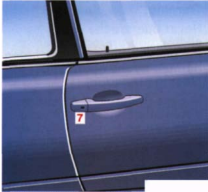
7 Infrared receiver in passenger door handle
