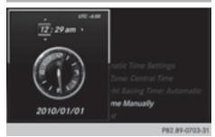
**Vehicles with GPS reception:** with manual time setting, you can set the time back or forward by up to several hours.
