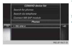
➤ To select a mobile phone from the device list: turn the controller and press to confirm.
