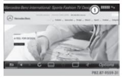
Display of existing connection and signal strength of the mobile phone network
