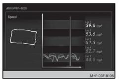
If Parameter is selected, the speed of the first five laps is displayed automatically.
